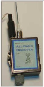
The Amazing All-Band Receiver is basically a diode detector followed by a high-gain audio amplifier. The detector uses a biased Schottky diode for excellent sensitivity and bandwidth; the detector will detect signals from below the AM broadcast band up to the microwave bands. The number of interesting signals is surprising; it is fun to drive around listening to the numerous strange sounds.
