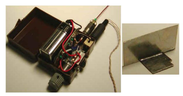
Any high-impedance high-gain audio amplifier circuit will work with the basic diode detector so feel free to experiment! Remember to leave the 10Meg bias resistor for the diode and couple the amplifier through a .01uF capacitor.
